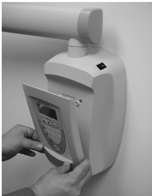
Figure 37 Snapping in the Operator Panel
