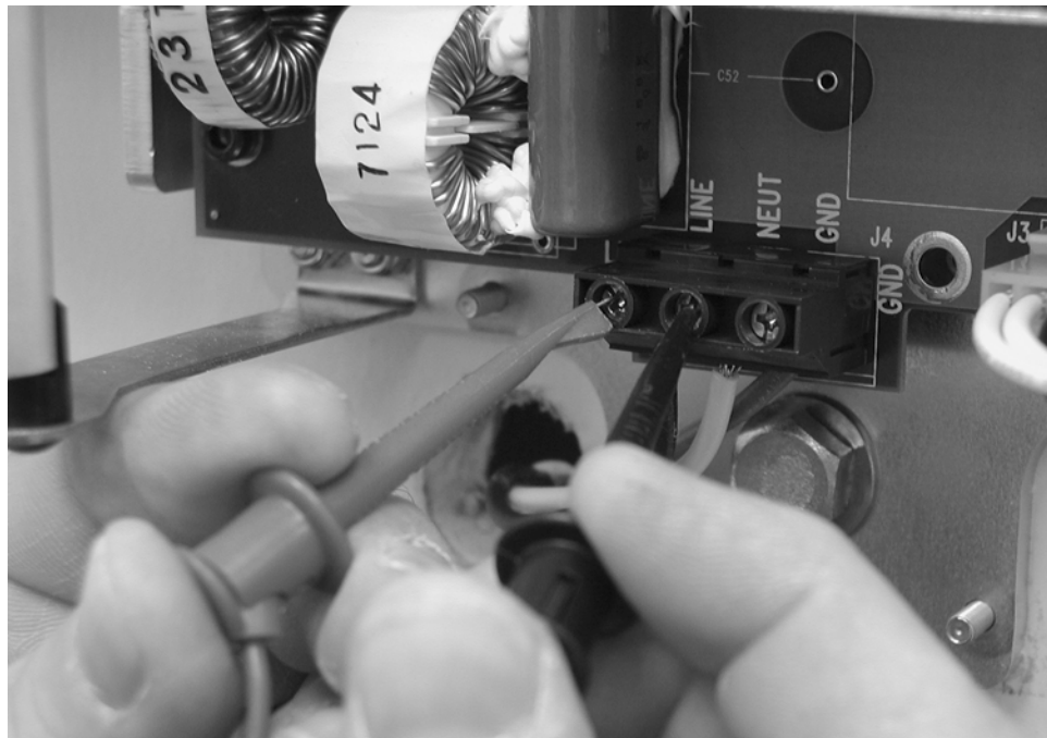
Figure 31 Verifying Input Voltage at the Line Input
