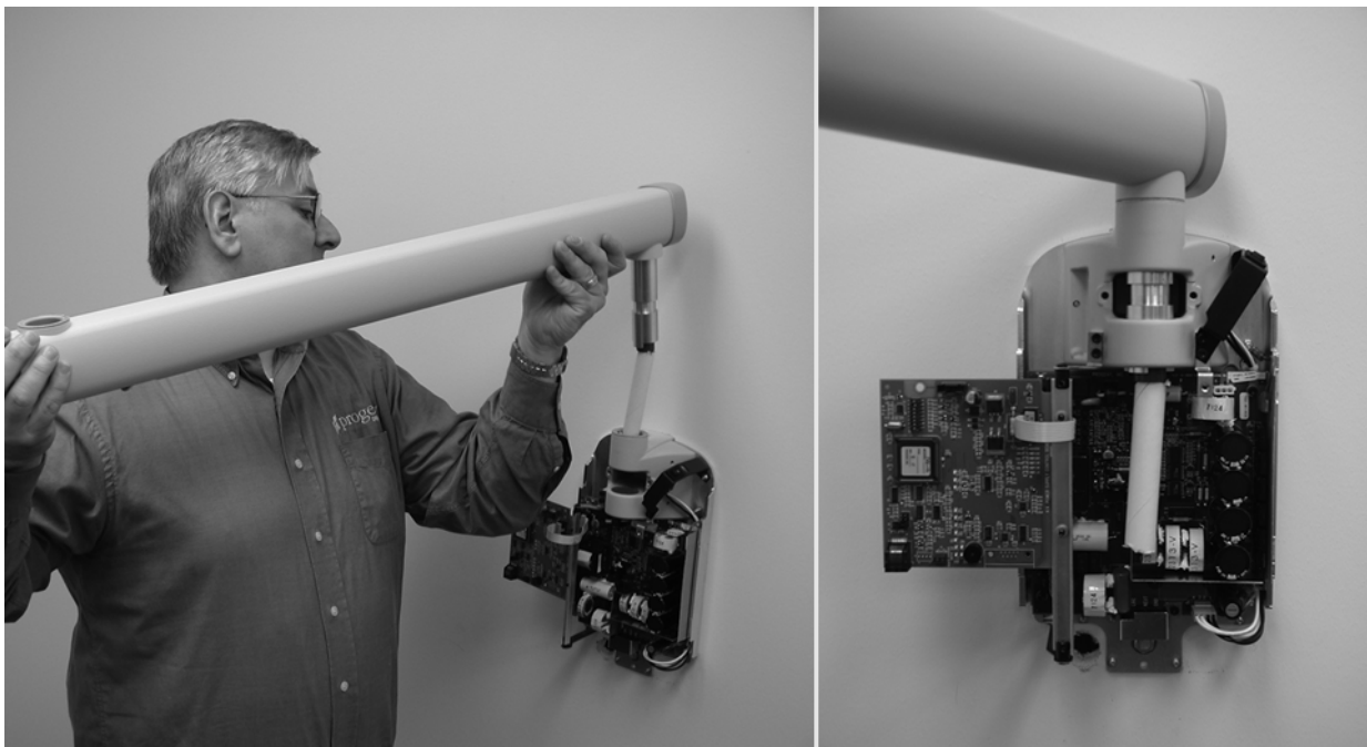
Figure 18 Installing the Horizontal Arm
